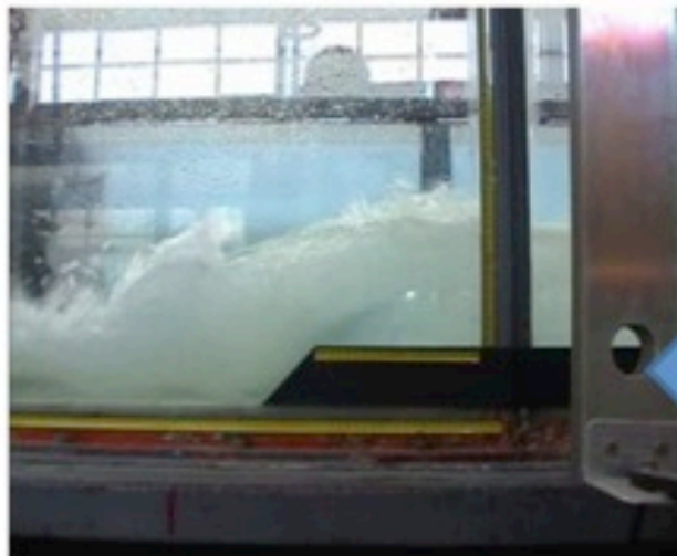
Physical model of a settling tank
